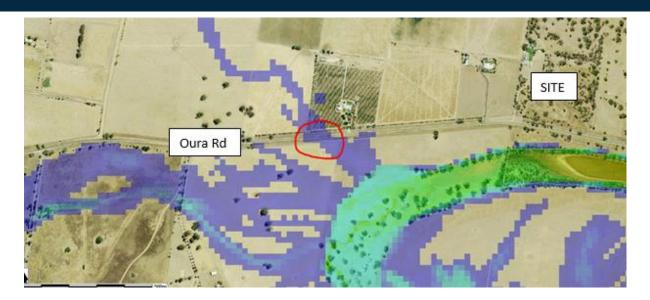
The flood model identifes that the road is cut at this location when the river guage height (at Hampden Bridge, Wagga) approaches 7.3m. A predicted river height reaching 7.3m at the Hampden Bridge guage would trigger an official "minor flood warning" from the Bureau of Meteorology which ranges from a river height of 7.3m to 9.0m for this guage.
